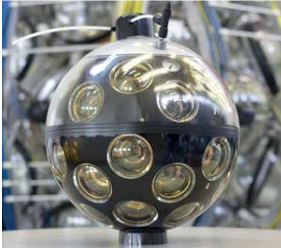
Fig. 2: A KM3NeT DOM consists of a spherical glass vessel with a wall thickness sufficient to withstand the enormous pressure at the bottom of the sea - up to 350 times the normal atmospheric pressure. In this glass vessel 31 photomultiplier tubes have been arranged to look in all directions for the faint light emitted by particles passing by.
