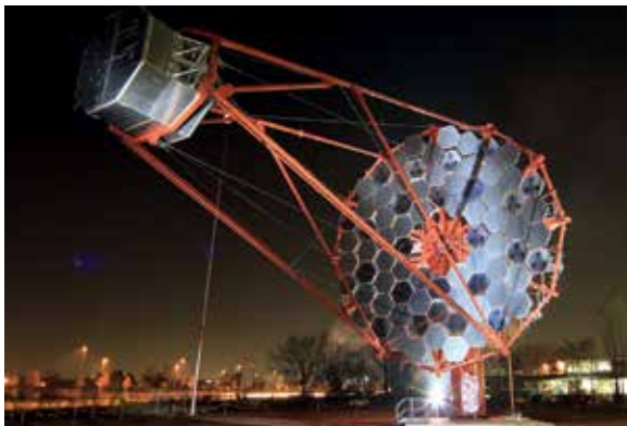
Fig. 2: Mechanical prototype of a CTA mid-size telescope in Berlin-Adlershof.
