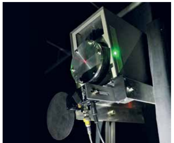
Fig. 2: The low-noise photomultiplier (in its cooling enclosure) used for the detection in the UV-extended visible range of photon wavelengths. The cross-section of the red and green laser beams marks the spherical center of the mirror.
